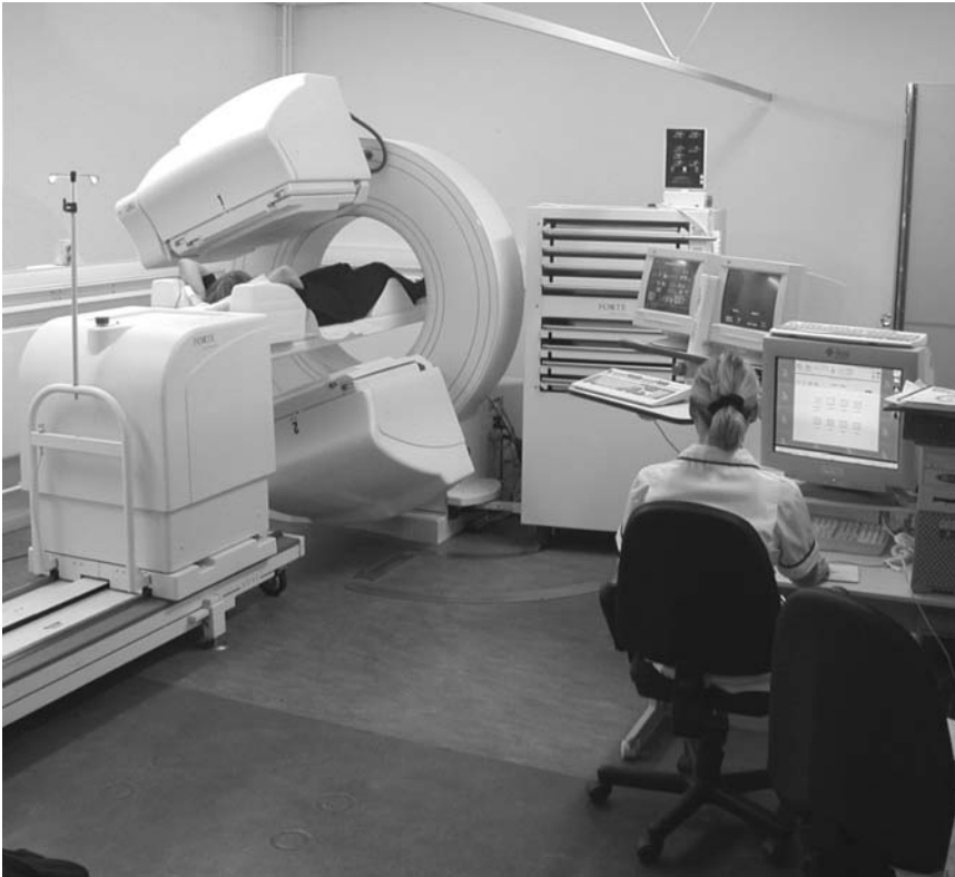
Figure 1.1. The gamma camera. The patient is lying between the detectors of this double-headed system. To the right of the camera is a rack containing extra collimators. The technician is seated at the computer controlling data acquisition and image display.
