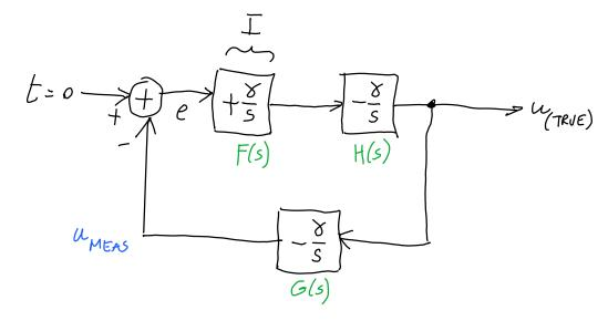
2. Find the open-loop transfer function, and find the phase margin. What does it imply about the stability of the closed-loop system?
