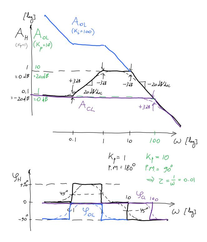
2. Find the closed-loop DC error, and phase margin, for proportional control with 20 dB gain.
