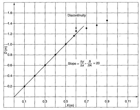
The discontinuity is probably caused by exceeding the limit of elasticity for this spring. Hooke's law assumes that the material is perfectly elastic and resumes its shape after being stretched or compressed:
