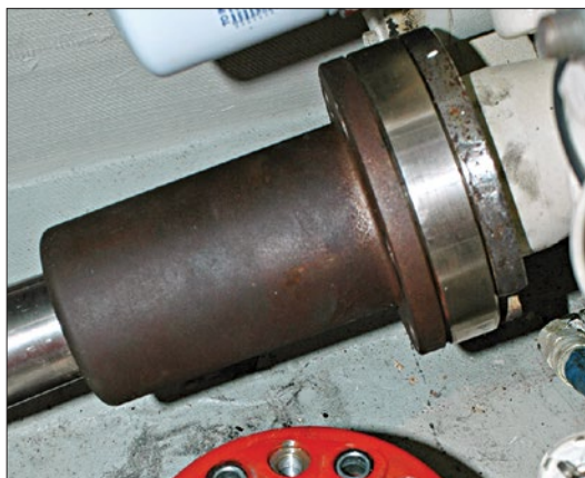
Above —This red nonmetallic coupling insert is designed to shatter if the prop strikes a large object. Insert surfaces lack the precision required for accurate alignment measurements. Before an alignment, the insert must be removed and the coupling faces brought together. If shaft length or the insertion of line cutters won’t permit that, a precision spacer like the one shown at left can be installed to perform the alignment.
