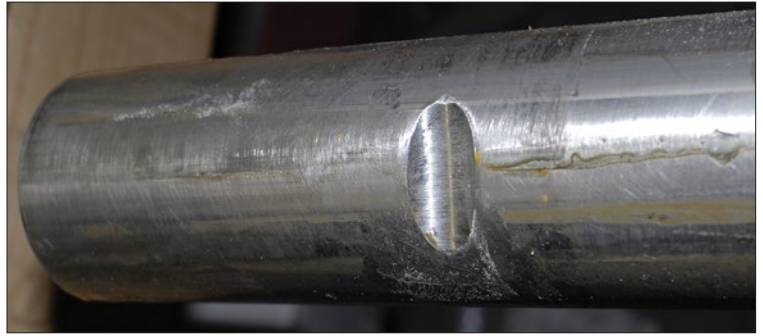
Left —Set screw tips should be either cupped or pointed, and hardened. Ordinary stainless steel fasteners, shown here, should not take the place of purpose-built screws. On the plus side, these set screws are secured with locking nuts and seizing wire. Above —Scallops cut into this shaft indicate that it's designed for use with a split coupling. Pinch bolts interface with the machined dimples to improve shaft-to-coupling engagement.
