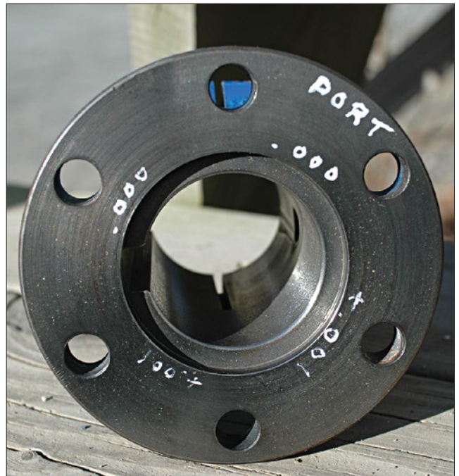
Left —Fitting and facing involves installing the coupling on its shaft and checking the coupling face's run-out. For correct alignment, the coupling face must be near perfectly perpendicular to the shaft centerline. If it's not, the face is milled on a lathe. Right —This coupling has been marked with its after-machining run-out, which does not exceed 0.001" (0.025mm).
