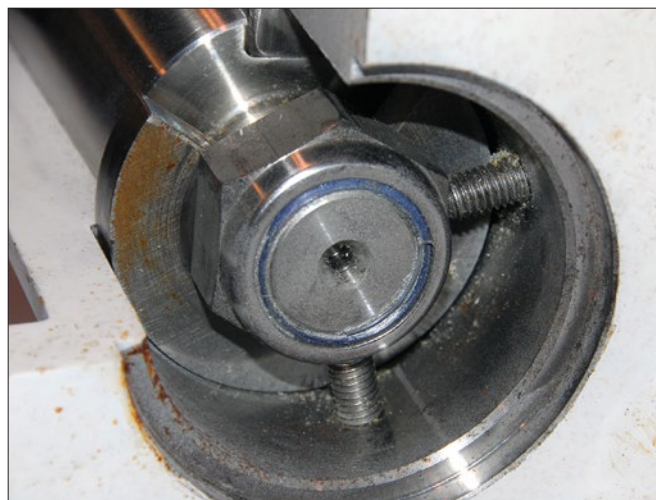
Left —Tapered couplings offer several advantages over straight and split models. The interface between the taper shaft and the bore makes for an exceptionally tight fit. In some cases where locking nuts have loosened, the shaft and coupling must still be separated with a hydraulic puller. Right —This tapered coupling has the added security of set screws to retain the locking nut.
