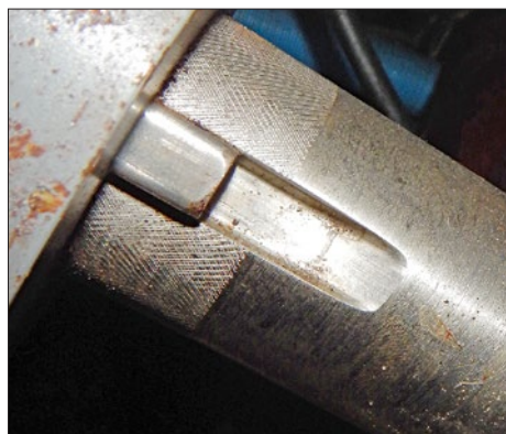
Left —A ramped and radiused keyway is more resistant to stress-induced fractures, while the knurling improves the interference fit on this small sail auxiliary straight-bore coupling. Right —Keys should fit snugly into a keyway and, when lightly oiled, should slide and be easily removed. Unlike this one, they should not rock or clack when moved from side to side.
