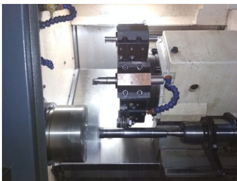
Figure 2 Experiment setup of roller burnishing process
