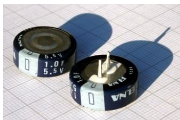
Fig 1 radial style and flat style super capacitor for electronics and mobile application
