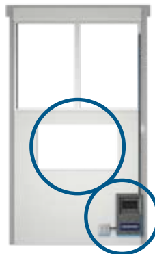
Layout with HVAC cutout & CB box
