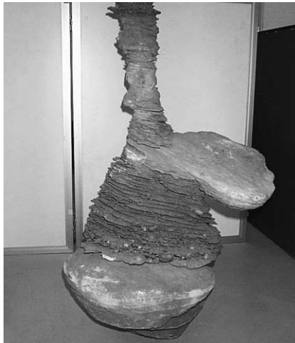
Figure 5.3 MEYCO® MP 301 injected into sand
