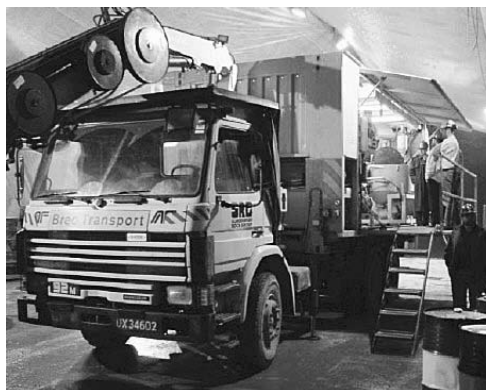
Figure 9.7 Container mounted multi-pump grouting system (AF Spesialprosjekt AS/SRG)
