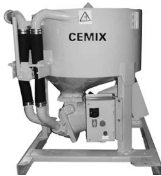
Figure 9.4 Typical colloidal mixer (Photo Atlas Copco)
