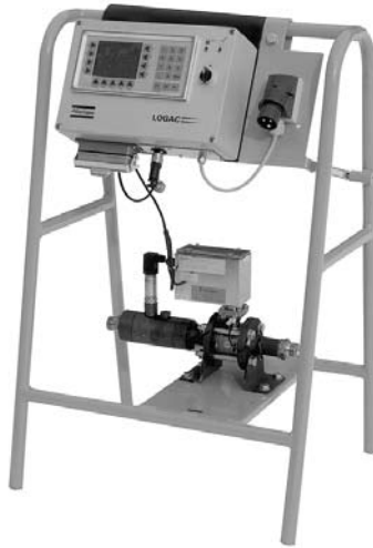
Figure 9.8 Example of a simple grout recorder (Photo Atlas Copco)
