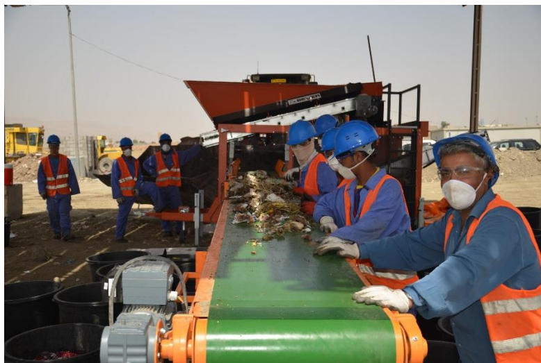
Figure 3: Materials recovery facility operating in northern Iraq – materials recovered or used in part as fuel for the LafargeHolcim Bazian cement plant. 25
