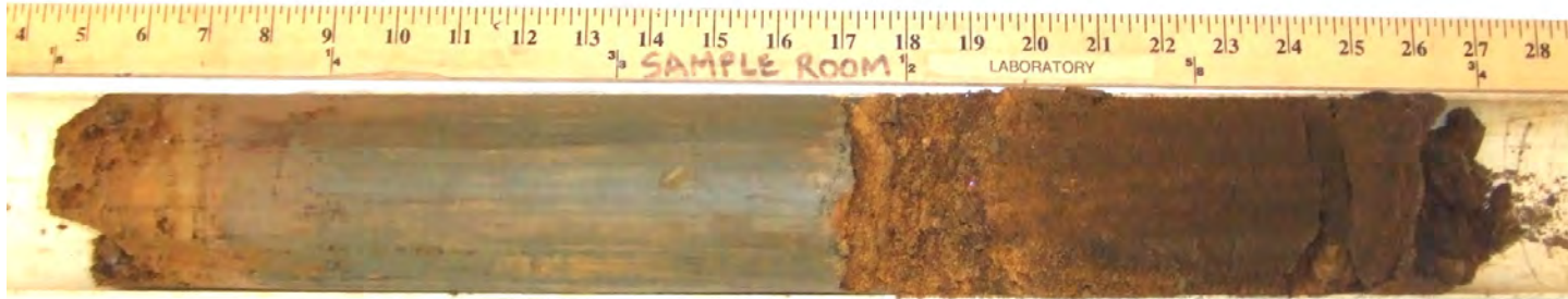
Figure 31. Shelby tube sample of Claryville Clay at its contact with the Old Licking River alluvium.
