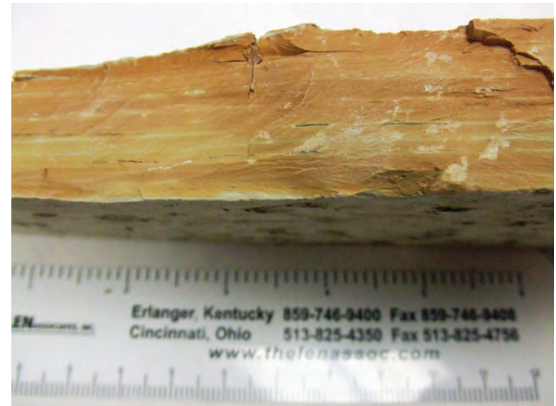
Figure 33. Burlington Group 2C lacustrine clays from basement excavation in Burlington, Kentucky. Note the pale blue silt partings that have been documented here and elsewhere in the Old Kentucky River valley (Ettensohn, 1974). Also note the fine laminae. These clays are highly plastic and can exhibit very high expansion potential.
