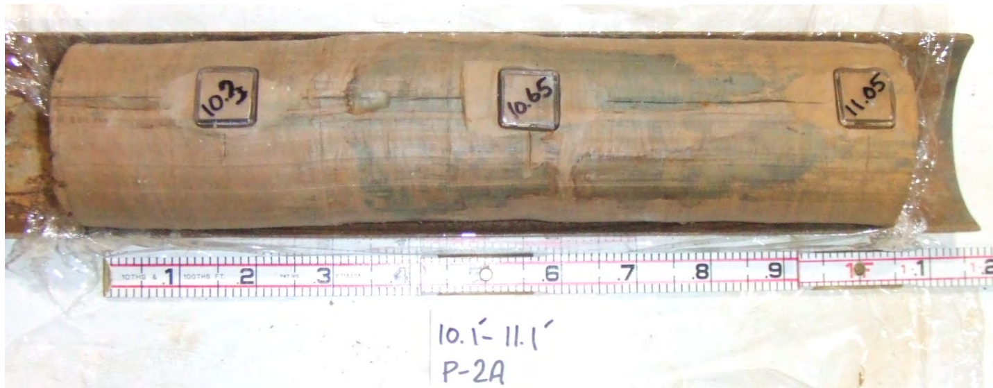
Figure 32. Oriented Shelby tube sample of Claryville Clay, obtained from a depth of 3.1 - 3.4 m (10.1 - 11.1 ft) from a site southeast of Alexandria, Campbell County, Kentucky (Fig. 30). Photo shows score line run down axis of sample during extrusion to mark the line of orientation. Remanent magnetism samples were obtained by pushing 12.7 mm x 12.7 mm x 12.7 mm (0.5 in x 0.5 in x 0.5 in), clear plastic boxes into the extruded Shelby tube sample at specific points along the scored line. Where necessary, the boxes were lightly driven into the sample using a rubber mallet. The top and bottom faces of the boxes were marked with permanent marker as the boxes were cut from the sample, and the lids were then placed on the boxes. The scale is graded in units of 3.05 mm (0.01 ft).
