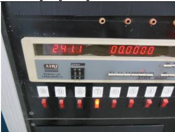
0.85times rating voltage running test
