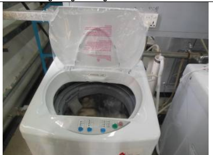
0.85times rating voltage running test
