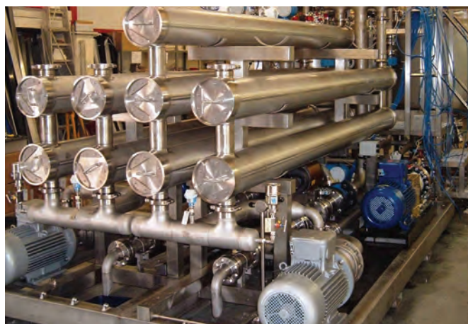
Hydra-Cell pumping for waste stream reduction and salt solution concentration at a pharmaceutical chemical plant.
