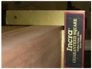
The goal of your jointer setup is to be able to make absolutely flat and square stock on two sides. Once two sides are flat and squared against each other, the planer can be used to enforce these angles on the other two sides.
