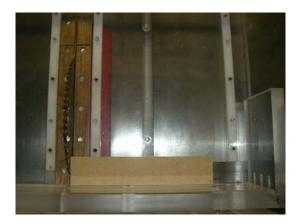
Once you remove the gauge blocks and move the stick over, the distance between the blade and the end of the block is exactly the same distance as the gauge blocks were:
