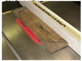
Step 3 – Resaw to .05" over nominal size (i.e. if your final size will be .500" thick, you will resaw to .550" thick). In this example I use a table saw, but band saw is also acceptable.
