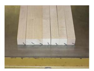
Step 7 – Now we will use the planer to enforce the known square corner onto the other two faces, while at the same time bringing the stick down to nominal thickness. You will plane each stick four times, once on each face. Because we are using squares, you will plane two edges, adjust the planer height, and plane the last two for your finished stock. You will turn the stick each time so that the angle is enforced according to the following chart:
