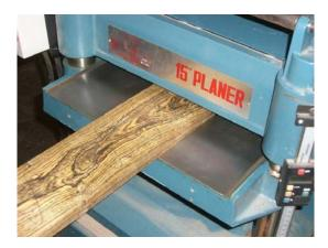
Step 5 – Now your stock should be parallel on the edges and faces. Your next step is to joint the edge one more time to ensure a square angle.
