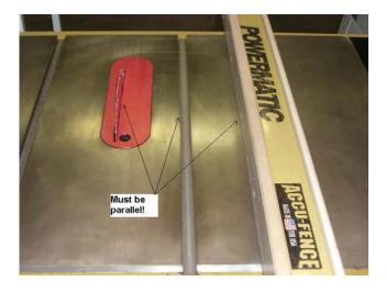
The fence should also be square to the tabletop, a measurement that is frequently overlooked. Finally, the blade itself should be set to exactly the angle you are trying to cut. Do not rely on the stops built into the saw – set the blade using a machinist square and make a cut, then measure the result and adjust accordingly.
