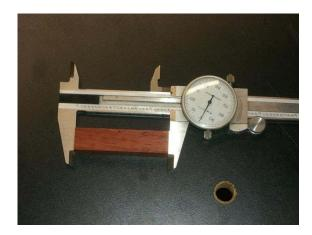
To achieve clean cuts, it is highly recommended to reinforce the back of the material with a disposable piece of wood so that the cut has zero clearance around the rear kerf. Finally, this is the time to double check that the blade is exactly square vertically, and that the fence is exactly square to the blade. As always, do not rely on the setup alone, but rather measure a sample cut to make sure you are achieving the desired results.
