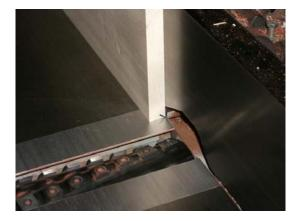
Now rip the stick from the plank, and go back and repeat the process until you have ripped the entire plank into sticks.
