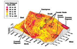
Figure 19.3 The use of remote sensing superimposed on totpography map to identify area that needed to be scouted. Remote-sensing layer is near infrared (NIR) band taken from airplane in 1997. Weed patches were identified by field scouting. (Courtesy: SDSU)
