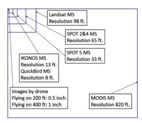
Figure 19.4 Different resolutions that can be collected by different sensors. (Dalsted et al., 2003)
