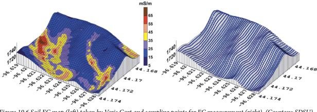
Figure 19.6 Soil EC map (left) taken by Veris Cart and sampling points for EC measurement (right). (Courtesy: SDSU)
