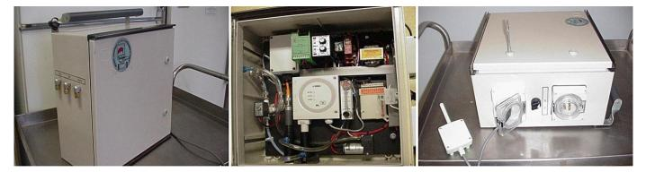
Figure 5 Environmental monitoring modules of the BASE-Q system<sup>[24]</sup>
