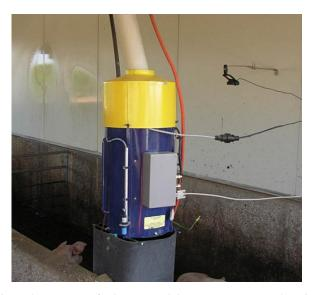
Figure 4 Prototype feed sensor and the camera system undergoing testing at a commercial piggery site<sup>[22]</sup>
