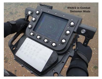
The battery life enables 1500 full discharge cycles and is recharged though an external recharging port on the RNAV2. Recharge time is <8 hours. The simple to operate ergonomic input devices and user-friendly mission planning software allow all levels of users to create waypoints and routes and easily upload them into the RNAV2.
