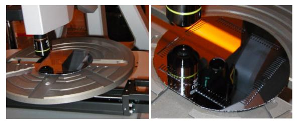
Figure 6.2 Wafer chuck and top CCD objective. The measurement coordinate system is indicated
