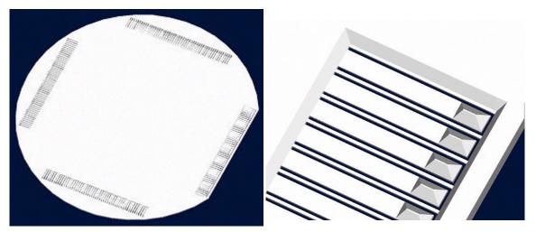
**Figure 4.7** Coupling array distribution on 4 inch wafer, notice the array orientation is in <110>
