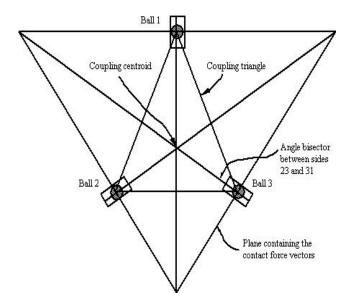
**Figure 3.3** Coupling arrangement to ensure stability (figure by A. H. Slocum, *Design of three-groove kinematic couplings* [9])
