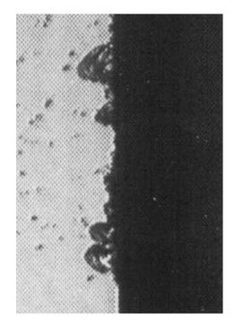
Figure 6.4 Detail of V-groove damage after M-1 & F1 wafer testing
