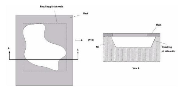
Figure 4.11 Silicon "pit" etched through wet anisotropic etch, using a concave cornered mask
