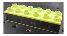
Figure 3.14 Lego<sup>TM</sup> block with aluminum sheet used as a target for the capacitive probes
