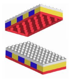
**Figure 3.16** Bottom and top view of the epoxied monolithic block used for the repetability vs. number of contact points bench level experiment
