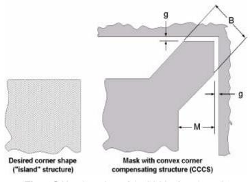
Figure 5.11 Dimensions of the CCCS, after Zhang [25]
