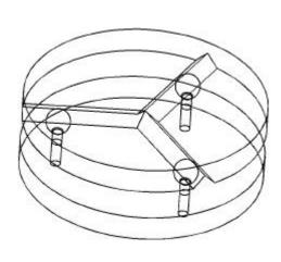
Figure 3.1 Three-groove kinematic coupling disassembled
