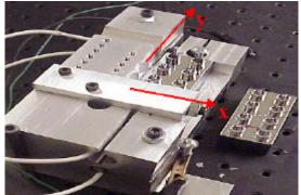
Figure 3.12 Font view of gauge block used to measure the repetability of 2x4 Lego<sup>TM</sup> blocks
