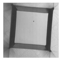
**Figure 5.3** Pyramid masked with CVD siliconnitride, shown after nitride strip. The low residual stress film yields sharp edges and smooth sidewalls after the KOH etch
