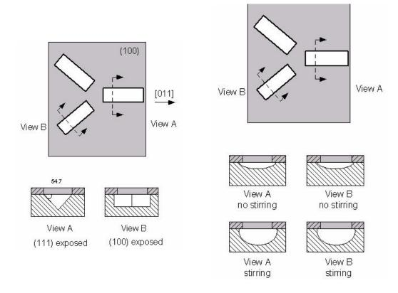
Figure 4.5 Anisotropic wet etch and mask
