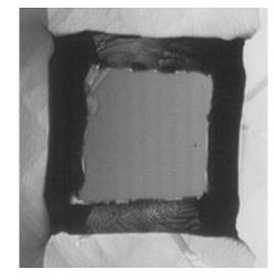
**Figure 5.2** Detail of stochiometric siliconnitride masked pyramid, showing jagged edges and rough surface finish
