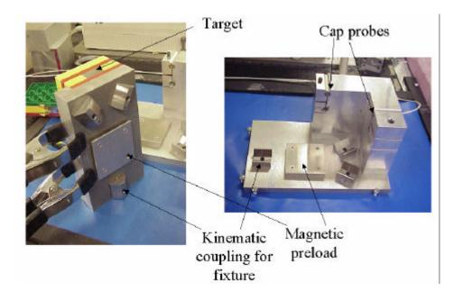
Figure 3.19 Experimental setup for the second bench level experiment
