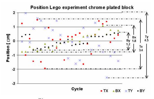
Figure 3.15 Lego<sup>TM</sup> block position in 30 cycle assembly-disassembly sequence, first bench level experiment
