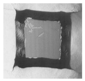
**Figure 5.1** Pyramid masked with stochiometric silicon-nitride, the thin film residual tress caused jagged edges and rough surface finish
