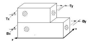
Figure 3.11 Measurement target for repeatability experiment of 2x4 PP Lego <sup>TM</sup> block
