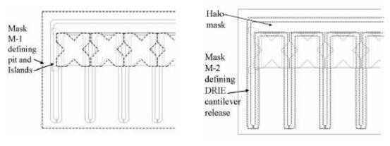
**Figure 4.14** Detailed view of Mask M-1 with overlapped Masks M-2 and F-1
