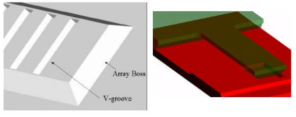
**Figure 4.9** Detail of concave coupling (V-groove) on boss
