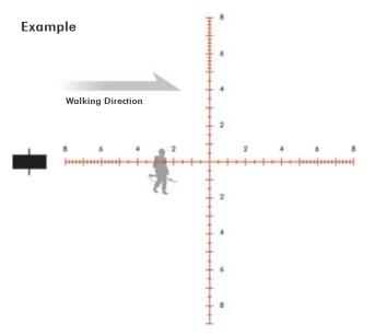
2.74 mrad correction for a man walking at 3 mph at 800 yards. No wind. Total bullet time of flight from trigger pull 1.5 seconds during which man travels 6.6 feet. Elevation already dialed into turret.
