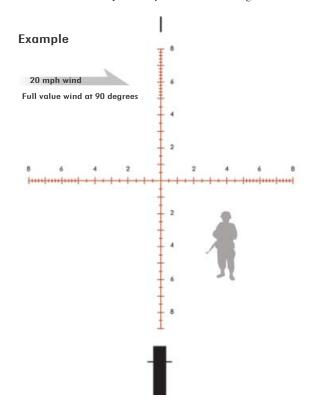
Using 3 mrad drop line at 500 yards, 4.0 mrad correction for 20 mph wind.
