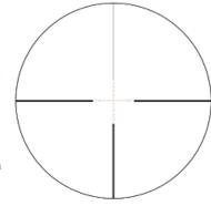
ensures that mrad specifications can be kept to the tightest tolerances possible. The fine center crosshair subtensions on the EBR-1 MRAD reticle were carefully chosen to provide the optimum balance between precision aiming and low light visibility.
