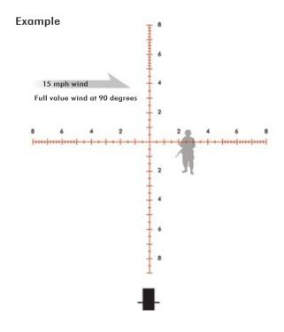
2.6 mrad correction for 15 mph wind at 700 yards. Elevation already dialed into turret.
