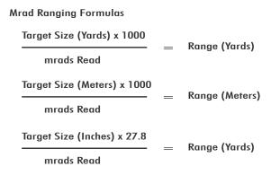
To use these formulas, you will need to know the measured size of the target or a nearby object. Using either the vertical or horizontal mrad scale, place the reticle on the target of known measurement and read the number of mrads spanned.
