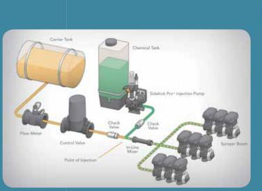
The Sidekick Pro injects chemicals directly into the in-line mixing tube to eliminate pre-mixing and costly leftovers.
