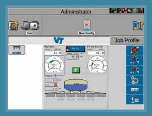
The Hawkeye System is built on the ISOBUS communication platform which allows it to work with ISO Task Controllers, including the Viper<sup>®</sup> 4.
