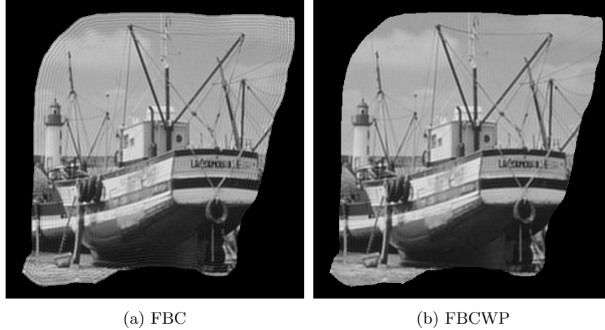
FIGURE 3. (a) The deblurred image by FBC from Figure 2(a). Those ripples are propagating into the center area as the iteration proceeds. (b) The deblurred image by FBCWP from Figure 2(a). The deblurred image shows no boundary artifacts at all. This result shows that FBCWP can deblur arbitrarily shaped images, without causing boundary artifacts.
