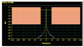
Figure 6. ISDB-Tb signal with no multipath or reflections.
