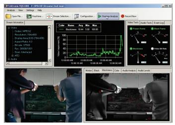
Figure 8. VQS1000 Blockiness graph peaking at 100% during a fast-action scene.
