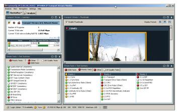
Figure 7. MTM400A measuring transport compliance from the ASI output of an RFM220.
