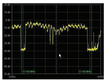
Figure 5. ISDB-Tb signal with poor frequency response. This signal has a digital carrier one channel below and a PAL signal one channel above.
