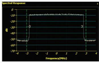
Figure 4. ISDB-Tb signal with good frequency response (no adjacent carriers).
