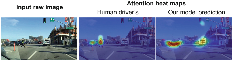
Fig. 1. An example of input raw images ( left ), ground-truth human attention maps collected by us ( middle ), and the attention maps predicted by our model ( right ). The driver had to sharply stop at the green light to avoid hitting two pedestrians running the red light. The collected human attention map accurately shows the multiple regions that simultaneously demand the driver’s attention. Our model correctly attends to the crossing pedestrians and does not give false alarms to other irrelevant pedestrians (Color figure online)
