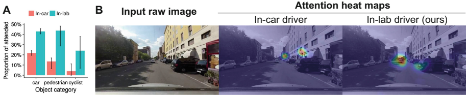
Fig. 2. Comparison between in-car and in-lab driver attention maps. (A) Proportions of attended objects of different categories for in-car and in-lab driver attention maps. In-car attention maps tend to highlight significantly fewer driving-relevant objects than in-lab attention maps. (B) An example of in-car driver attention maps showing irrelevant regions. The in-lab attention map highlights the car in front and a car that suddenly backed up, while the in-car attention map highlights some regions of the building
