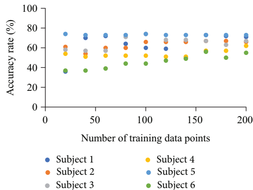
FIGURE 12: Prediction result for minimum toe clearance using 100 test gait data (accuracy rate).
