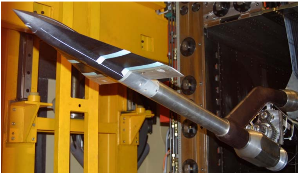
Figure 2: 65°-swept delta-wing-fuselage-model-configuration with remote controlled trailing-edge flaps on the roll-rig device in the DNW-TWG Göttingen.
