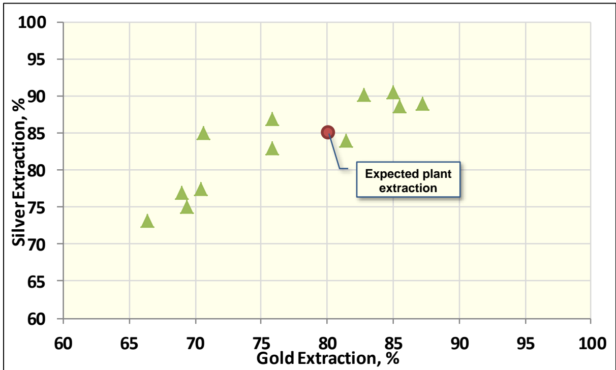
Figure 16.3: Whole Feed Silver Leach Extraction vs. Gold Extraction (2013 Test Results)
