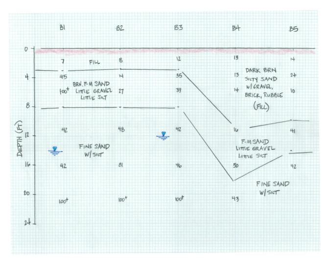
Fill was encountered at all the test holes to depths of  $\approx$ 3-10 ft. Deeper Fill was encountered at B4 & B5. The Fill varies in composition but generally consists of a dark brown, Sand, little gravel, little silt.. Trace amounts of rubble, loam and other matter are embedded in the Fill. The Fill varies from loose to medium dense. Fill should also be expected around existing foundations and utilities.
