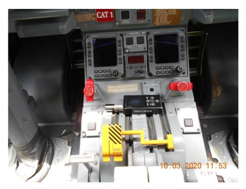
Figure 3: Position of engine number 1 fire handle at post occurrence inspection
