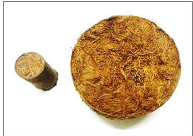
Figure-1. The prepared Kenaf sample with natural rubber binding.
