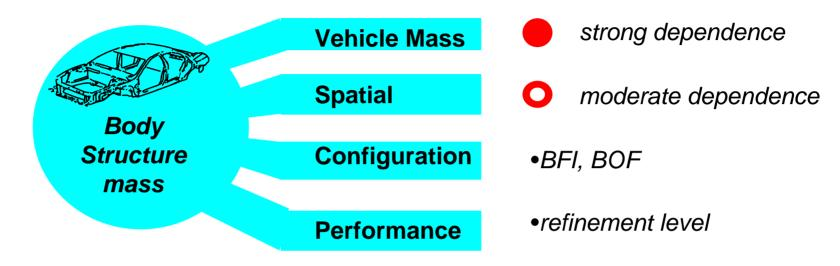
subsystem mass = f (gross vehicle mass, vehicle area, configuration, performance)
