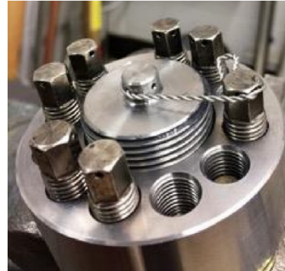
Figure 10.—Supernut-separation bolt safety wire configuration using proper horizontal alignment and correct winding direction around center post.
