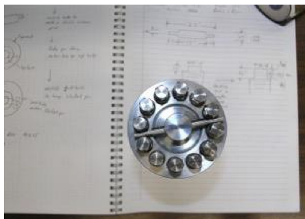
Figure 18.—Bladed cotter pin used for positive locking of supernut-separation bolt.
