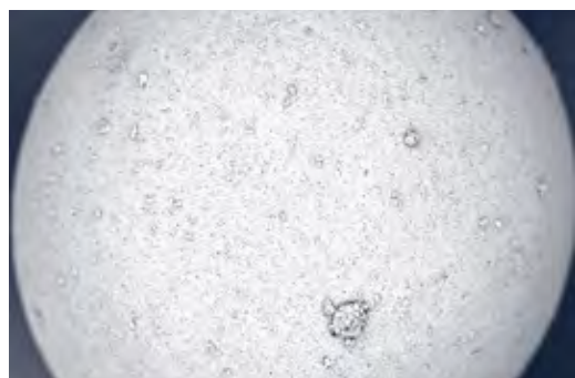
CT 3000 SDP: Spray dried powder granule
