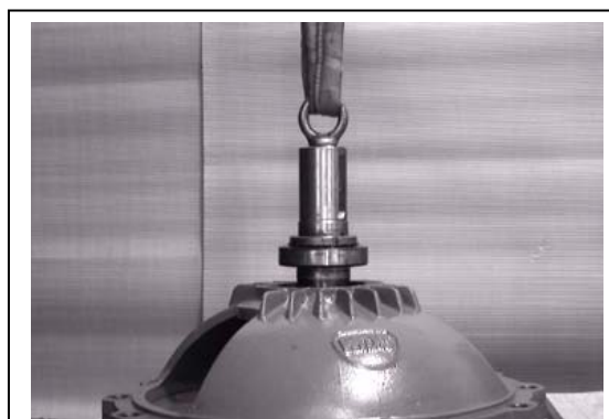
Fig. 6 Removing shaft unit
