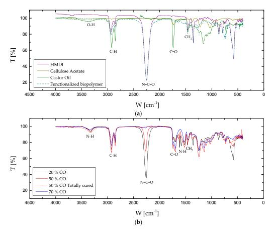
**Figure 1.** Fourier transform infrared spectroscopic attenuated total reflectance (FTIR-ATR) spectra for: (a) 1,6-hexamethylene diisocyanate, cellulose acetate, castor oil and functionalized biopolymer; (b) formulation with 20% CO, 50% CO, 70% CO and 50% CO totally cured.
