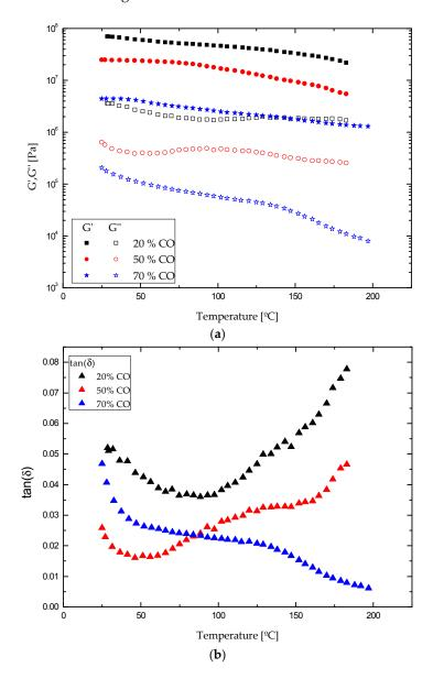
**Figure 8.** Temperature ramps for all ecofriendly bioadhesives at 2 °C/min of heating rate within the linear viscoelastic region: (**a**) elastic (G') and viscous (G'') moduli; (**b**) loss tangent (tan $\delta$ ).
