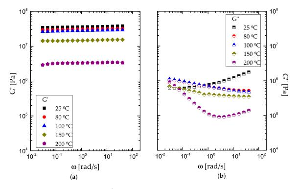
**Figure 5.** Evolution of (**a**) elastic, *G*′, and (**b**) viscous moduli, *G*″, with frequency, within the linear viscoelastic range, for formulations containing 50% CO castor oil at different temperatures.
