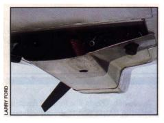
The cowl exit area was reduced by 70% to cut cooling drag.
