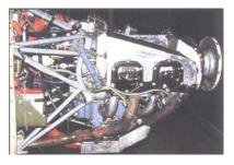
N402C uses a 160 hp Lycoming with a tuned crossover exhaust system.
