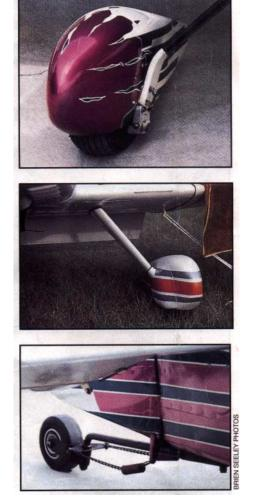
N402C's main gear fairing (top) and nonfaired tailwheel (bottom). The center photo shows a Mustang II with stall strips and brake fairings.
