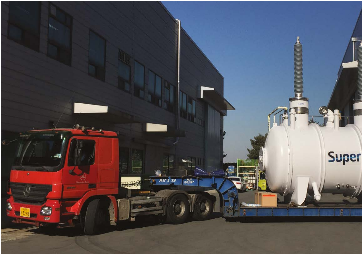
Figure 3. One phase of SuperOx 220 kV SFCL in KERI test centre, February 2018
