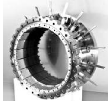
Figure 30: "Porcupine" ferrite-lined beam pipe HOM load of the CESR B-cell cavity [40].
