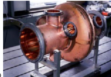
Figure 5: Cavities for high-current storage rings. (a) 500 MHz CESR cavities, (b) 508 MHz KEKB cavity, (c) 400 MHz LHC cavity.
