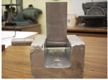
Pivots Nicely Photo by R. G. Sparber The clapper easily swings up. It flops back down with a slight push. All that is left is to trim the pivot pin.
