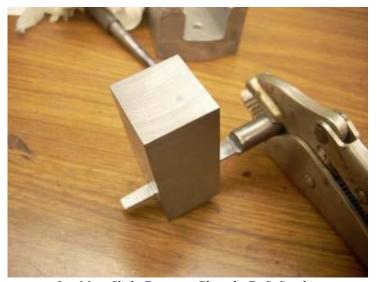
One More Slight Ream Photo by R. G. Sparber It was then a simple matter to use the reamer to gently remove a tiny amount from just the clapper's hole.
