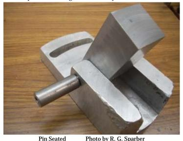
Pin Seated Photo by R. G. Sparber It turned out that the minimum diameter of the pin was larger than the minimum diameter of the hole! A quick pass with a <sup>1</sup>/<sub>4</sub>" drill and the pin went in all the way.
