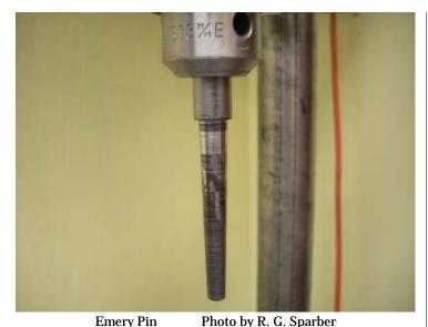
Before I did any damage, I blued the pin and wrung it in the hole.
