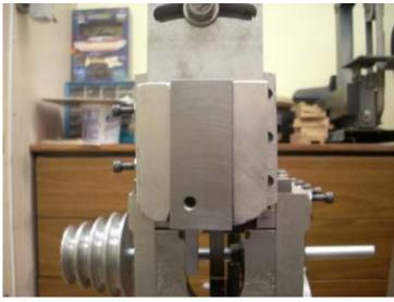
Clapper Set Screw Hole Photo by R. G. Sparber His design places the cutter on the center line of the pivot pin in order to minimize chatter.
