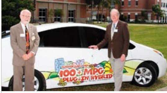
At the forum, Frank Leslie, adjunct professor in the Department of Marine and Environmental Systems at left, and Dean of the College of Science Gordon Nelson, pose by a Prius modified to become a plug-in hybrid. A third-party manufacturer, the Hymotion Co., modified the car. Charged by a normal 120-volt house utility outlet, the car's battery will take it 40 miles, which is adequate for typical in-town travel. When the voltage falls to a certain level the gas-powered engine automatically starts and recharges the battery.
