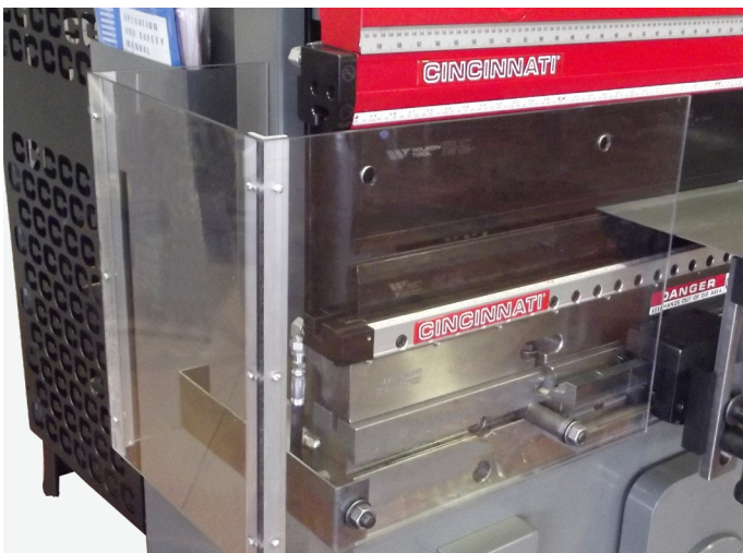
End barrier and front-mounted partial barrier safeguard the ends of these full length dies.
