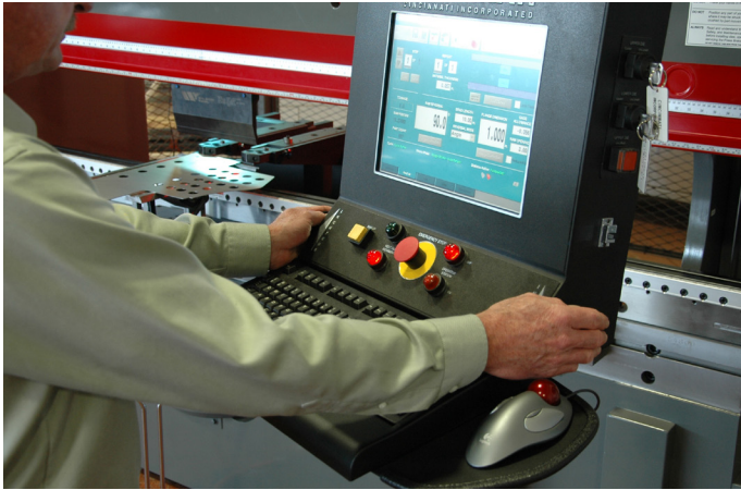
The operator activates the press brake using the dual palm buttons.
