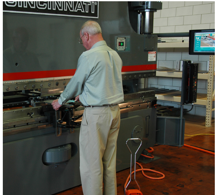
The operator loads the workpiece. NOTE /// Blanking is used to accommodate the use of material support arms.
