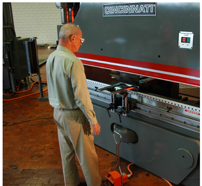
The workpiece has moved up through the sensing field during the forming operation. The “Mute” adjustment was ON to allow this and a corresponding “Guard Off” warning light is ON alerting the operator of the status of the safeguard.
