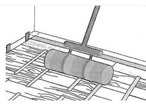
Use 100-150 lb. roller to apply pressure to installed sections while the adhesive is still active (approximately 45-60 mins).
