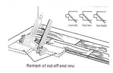
Use manual or pneumatic nailer for subsequent rows. Each plank should be nailed every 6". Fasten each plank with at least 2-nails. Do not nail less than 2" from plank end to prevent the tongue from splitting.
