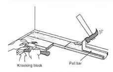
Cut plank to fit end row, allowing for 1/2" expansion gap and fasten with pull bar.
