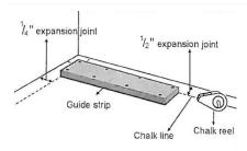
Use chalk line to trace starting line with W' expansion joint at the side and Y." at row end. Nail the guide planks along the starting line. The plank will serve as a guide for the 1st row of plank.
