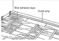
Use blue adhesive tape every five or six rows to ensure planks remain firmly in place.
