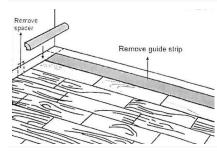
Remove the expansion spacer to install molding to cover the expansion joint
