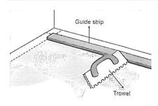
Use the trowel and apply adhesive at a 45° angle from the starting line outward.
