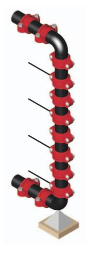
When using flexible couplings, the movement that occurs in long lengths of piping needs to be considered. Each joint can move up to the maximum pipe end separation published. This movement can accumulate and result in the growth of the piping system, for example at the top. Offsets may be necessary.
