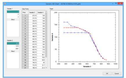
Figure 4: Piping Design Tensile Strength Table for ASME B31.3 Calculations for ASTM A106 Gr B Material
