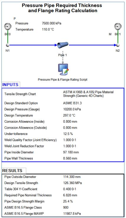
Figure 1: Example Flownex Pressure Pipe Network with Script
