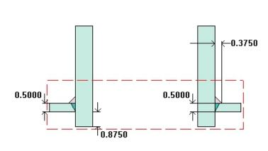
$$\begin{array}{ll} t_{w(lower)} = & 0.5 \text{ in} \\ Leg_{41} = & 0.375 \text{ in} \\ Leg_{43} = & 0 \text{ in} \\ h_{new} = & 0.875 \text{ in} \end{array}$$
