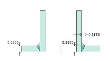
$\begin{array}{ll} t_{w(lower)} = & 0.68 \text{ in} \\ Leg_{41} = & 0.375 \text{ in} \end{array}$
