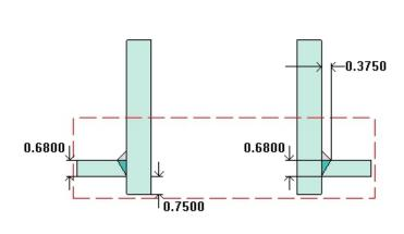
$\begin{array}{ll} t_{w(lower)} = & 0.68 \mbox{ in} \\ Leg_{41} = & 0.375 \mbox{ in} \\ Leg_{43} = & 0 \mbox{ in} \\ h_{new} = & 0.75 \mbox{ in} \end{array}$
