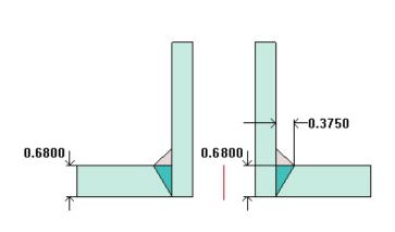
$\begin{array}{ll} t_{w(lower)} = & 0.68 \text{ in} \\ Leg_{41} = & 0.375 \text{ in} \end{array}$
