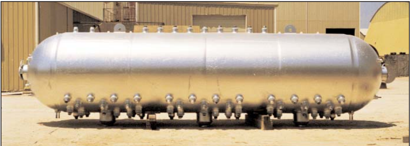
Sec. I Steam Drum, 65" ID x 3.5" w x 43'-7" s/s, weight 140,000 lbs. with (103) 4" riser tube conns. TFES can provide process design and fabrication responsibility for all steam drum internals or install our customers' designed internals.
