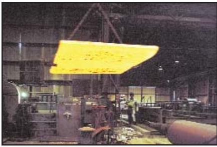
Five (5) pyramid and pinch plate rolls can roll plate hot or cold and up to 7.5" thick. Roll lengths vary up to 16'.
