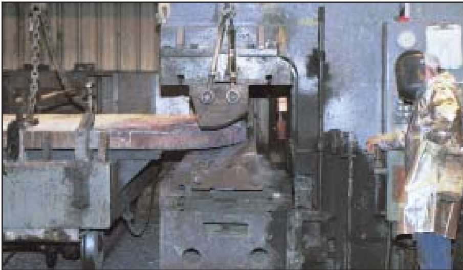
Plate rolling roundness and efficiency is enhanced by the use of the crimping process prior to rolling. Crimping sets the correct radius on the ends of the plate and eliminates the waste of excess material.
