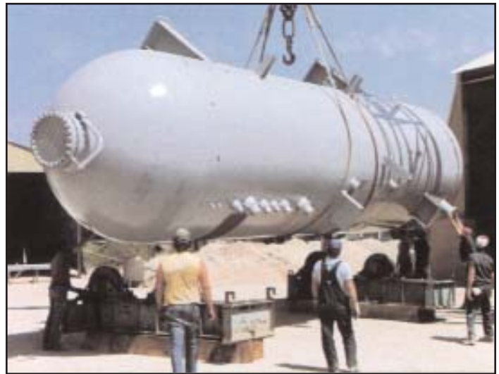
Supercritical CO2 Reactor, 114" ID x 3" w x 31'-0" s/s, weight 148,000 lbs. Overlayed with 316 SS.
