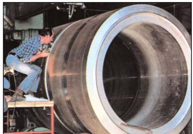
The strip overlay process is used on heavy wall vessels like reactors, requiring alloy internal surfaces. The strip overlay method is a submerged arc process, resulting in controlled chemistry and a high integrity bond.
