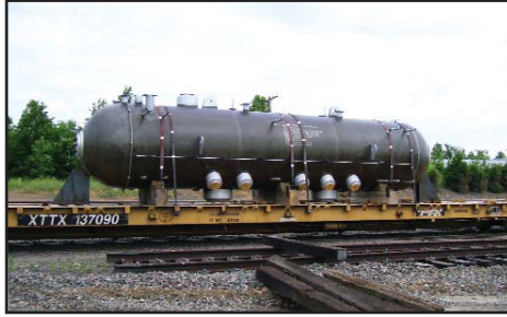
Pressure Vessels (Steam Drum)
