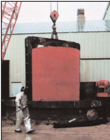
Extensive heat treating facilities at Taylor Forge allow special metallurgies to be quenched and tempered. The large stress relief oven gives in-house post weld heat treat capabilities up to 15' diameter.
