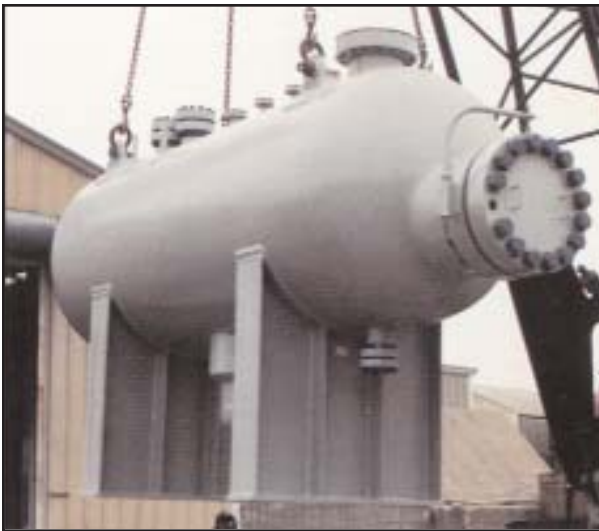
Suction Scrubber, 69" ID x 5.25" w x 22'-0" s/s, weight 92,000 lbs., 2500 psi design. Offshore platform, Malaysia.
