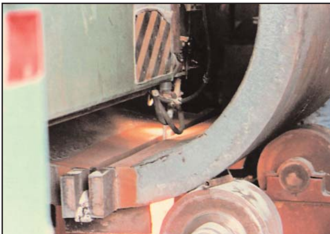
After the plate is formed into cylinders, many welding processes are used to fabricate the rest of the vessel. Here a submerged arc procedure is used for a longitudinal seam.
