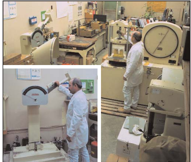
In-house laboratory for destructive testing procedures including Tinius-Olsen tensile machine for tensile tests and weld bends, Tinius-Olsen Charpy impact machine, Rockwell hardness machine, and Brinell hardness machine.
