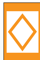
DANGER! Nature of danger may be indicated inside the diamond shape such as rocks, shoals, dams, construction, or stumps.
