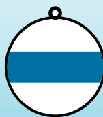
MOORING BUOY White with reflectorized blue band. May have white light or reflector.
