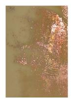
Fig. 10 Etched fingerprint remaining on PCB
