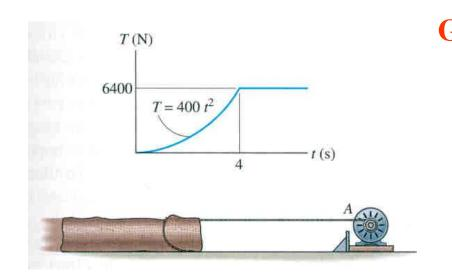
Given: The 500 kg log rests on the ground (coefficients of static and kinetic friction are  $\mu_s = 0.5$  and  $\mu_k = 0.4$ ). The winch delivers a towing force T to its cable at A as shown.
