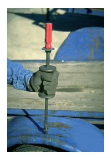
A dent in an automotive fender can be removed using an impulse tool, which delivers a force over a very short time interval.
