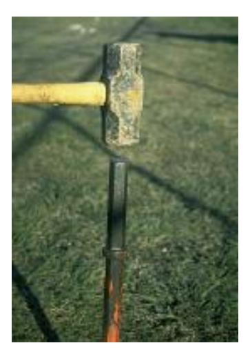
Sure! When a stake is struck by a sledgehammer, a large impulsive force is delivered to the stake and drives it into the ground.
