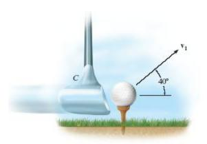
Given: A 40 g golf ball is hit over a time interval of 3 ms by a driver. The ball leaves with a velocity of 35 m/s, at an angle of 40. Neglect the ball's weight while it is struck.
