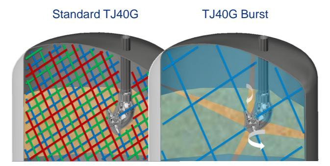
Less caustic is necessary to wet the tank surface using TJ40G Burst as there is no need to build up a dense cleaning pattern
