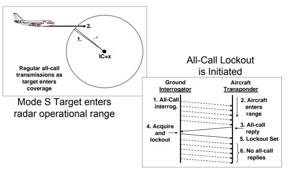
Figure 2. Stages of Lockout
