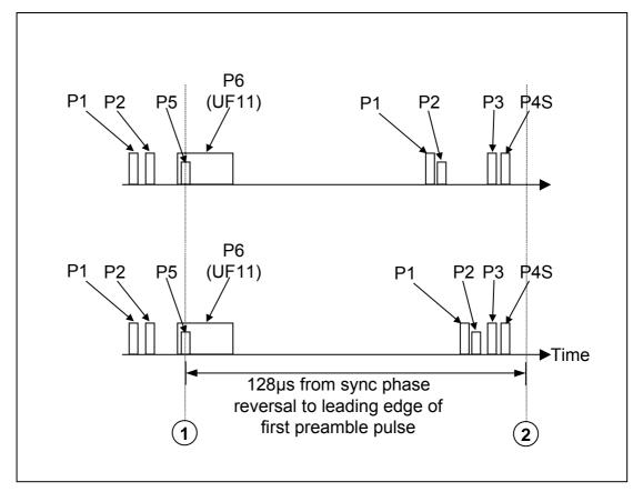
Figure 9. Combination of Mode S and Mode A/C in Same All-Call Period
