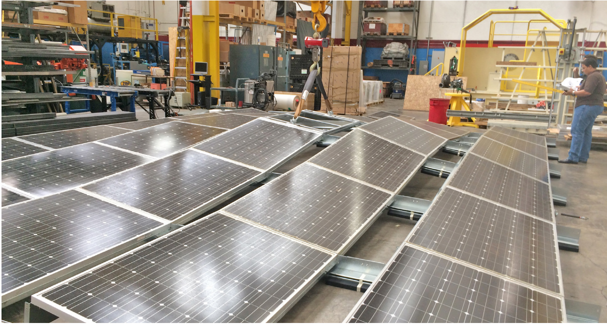
Figure 3: Empirical Testing to determine load sharing values (Photo Courtesy of DCE Solar)
