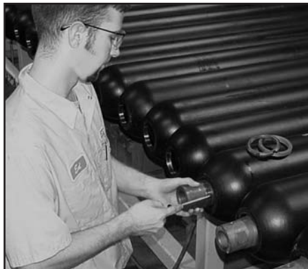
Assembly of bladder accumulators
